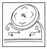
Vehicles with outside power mirrors have the controls on the driver door armrest.
